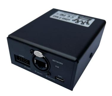
Power over Ethernet 802.3af / network 10/100Mbps RJ45 Ethercon socket. USB-C socket for DC power input alternative to PoE. 10way IDC socket for I/O triggering. See eDMX MAX Recorder Manual.
