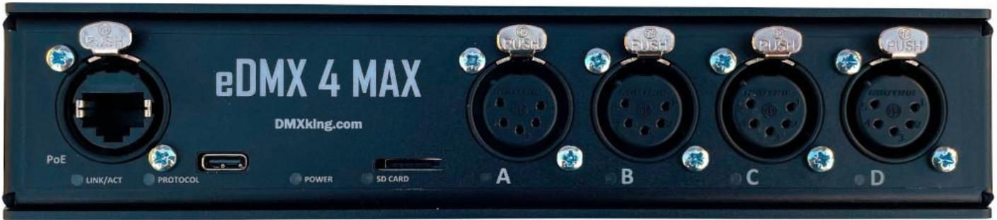
Power over Ethernet 802.3af / network 10/100Mbps RJ45 Ethercon socket. USB-C socket for DC power input alternative to PoE. SD card push-push socket for microSD. Four Neutrik XLR connectors for DMX512 3pin or 5pin options available.
