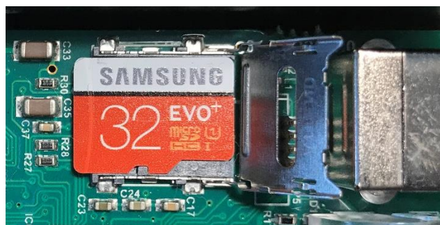
MicroSD card placed on holder – line up the notch
