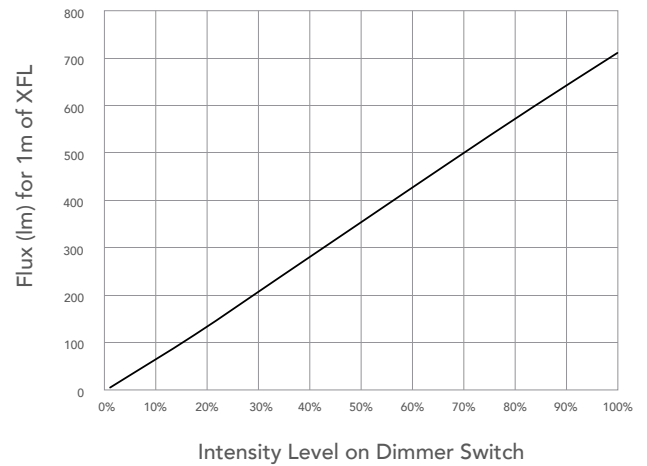
XFL DW 4000K-2200K, Flux vs Intensity Level
