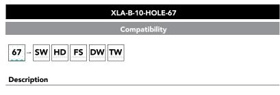
IP67 end cap or boot with hole, for 10mm strip.
