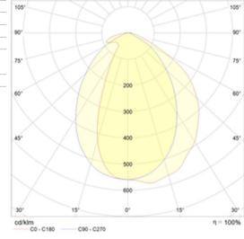
Wide beam asymetry optimised for stairs and walkways for homogenous light.
