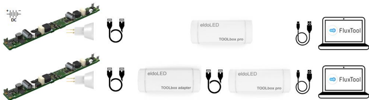
Figure 9: The 32W/P LED driver is fully programmable via FluxTool. If the 32W/P LED driver is already powered by a DC PSU, only TOOLbox pro is required (top). If the 32W/P LED driver is not powered, programming can be done with TOOLbox pro in combination with TOOLbox adapter (bottom).
