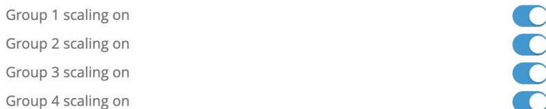
Figure 8: LED outputs can be set to “active” or “inactive” via the Group Scaling settings in the Control section of FluxTool. Best practice is to set any LED output, which is not connected to an LED load, to “inactive” to ensure optimal LED driver performance. In this example, all LED outputs are set to “active”.
