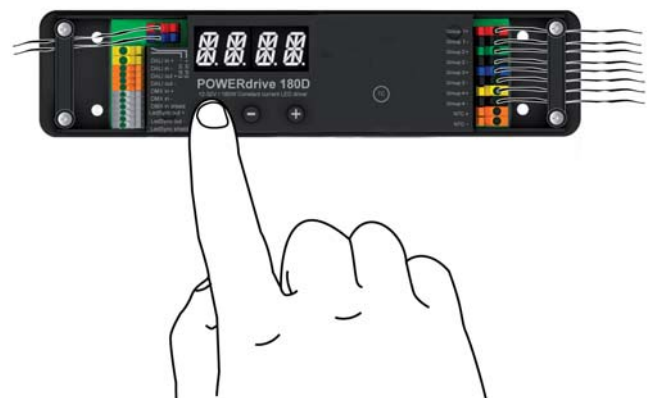
G Configuring the POWERdrive
