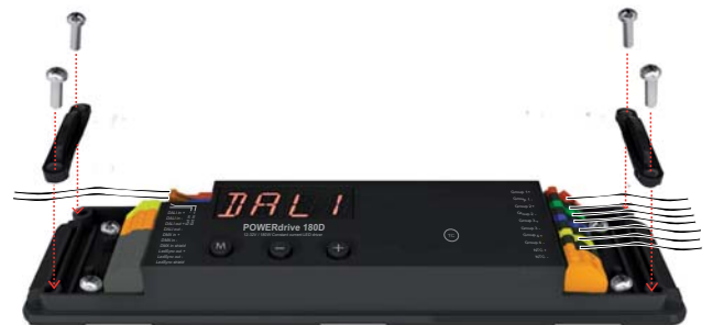
F Fastening the strain reliefs
