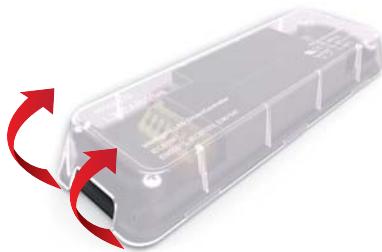
A Removing the cover
