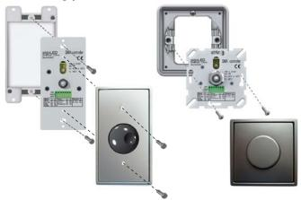
The DIP switches remain accessible after installation. When carrying out changes in the DIP switch settings, turn the DimWheel off and on again (by pressing the knob twice) to activate the new settings.
