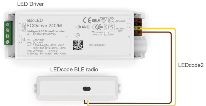
Wiring diagram BT-L2C1
