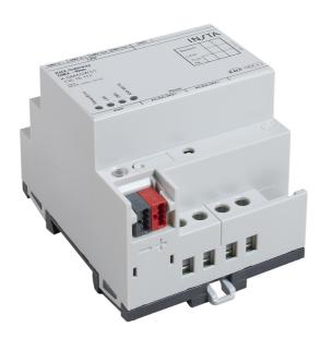
Intelligent system device, RMD-type, for coupling of DMX512 systems to KNX. To this effect, the KNX Gateway DMX-Web is connected to the KNX and the DMX512-bus. The gateway requires AC/DC24 V supply voltage.
