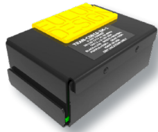
Above: Eulum TRAN-XIT translates Bluetooth to standard 1-10V signals.
