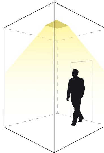
Motion detected: light output is increased to 100%
