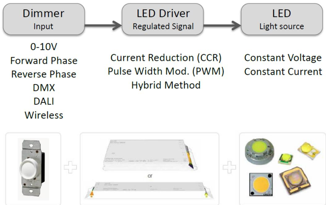
The images below describe the pros and cons of different LED dimming methods. Their usage is dependent on manufacturers' preference if not specified. PWM is typically most cost-effective so it is most often used.
