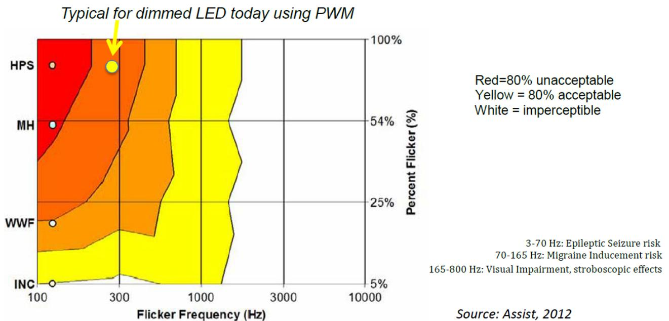
A luminaire should be in compliance with the characteristics below to be considered flicker free.
